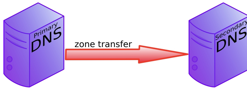
Figure 7.3.: Zone transfer from a primary to a secondary name server
